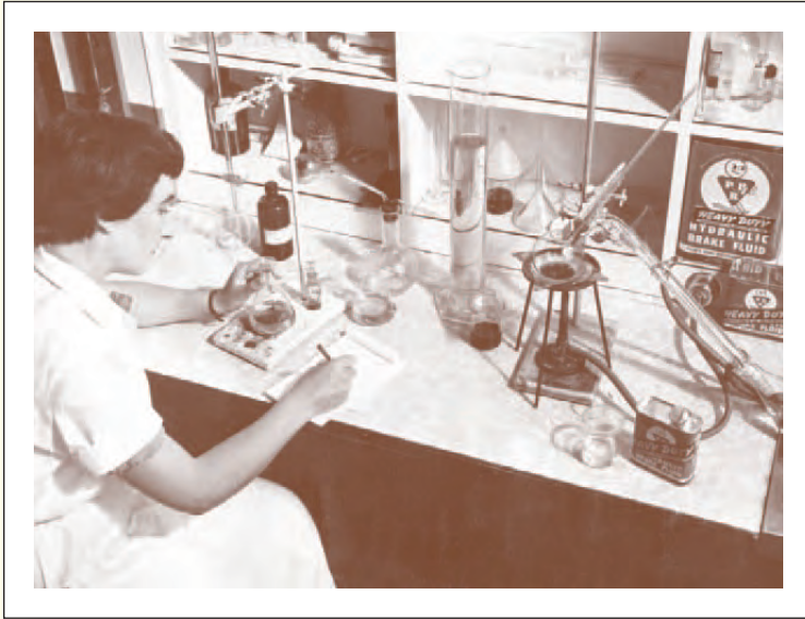
For many years, PBR sold its own brand of brake fluid which had a higher boiling point than fluid imported from overseas. Here brake fluid is being quality tested in the PBR laboratory.
